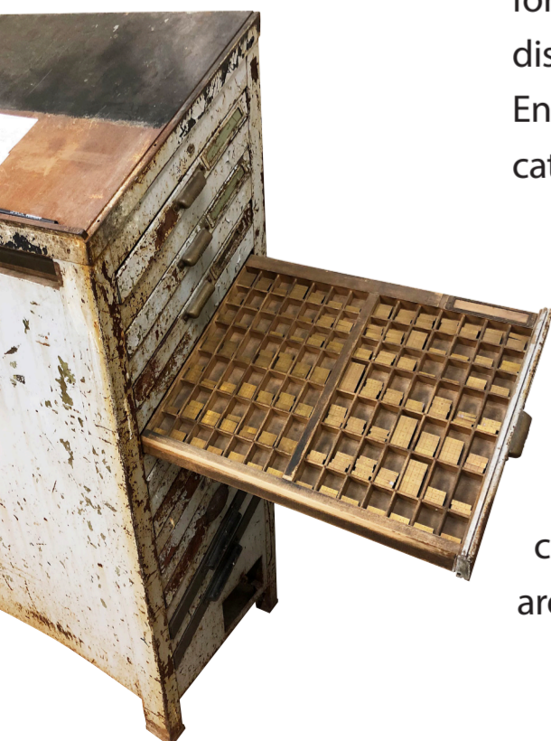
Ludlow Matrix cabinet, Angle Top model.
