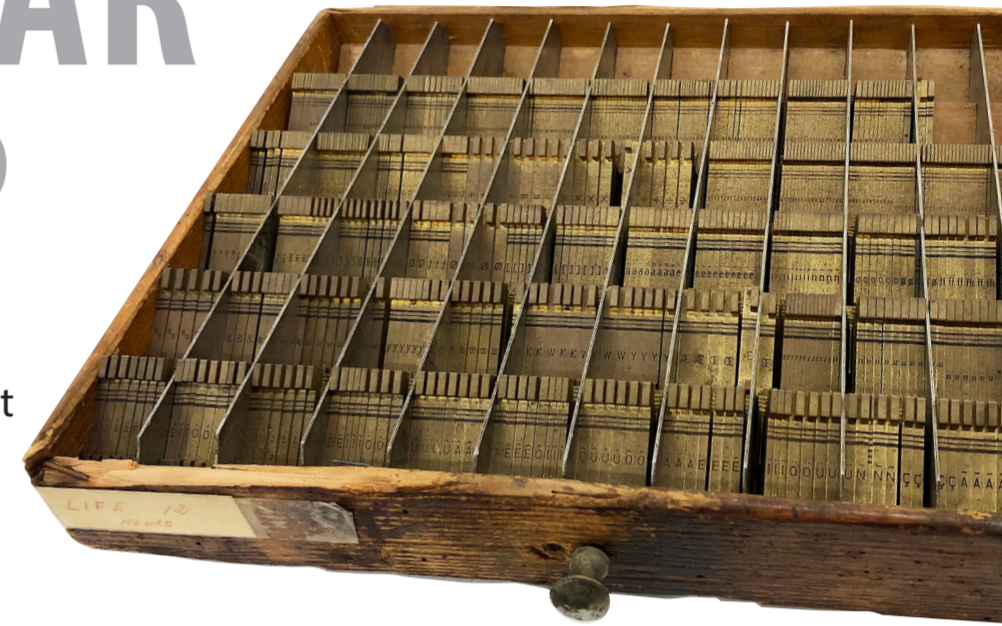
Cabinet drawer with Linotype matrices of Life roman and italic, 6 pt body.
